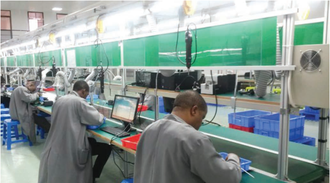
Workers assembling pre-paid electrical energy meters at the Inhemeter Tanzania Limited factory in Dar es Salaam.
